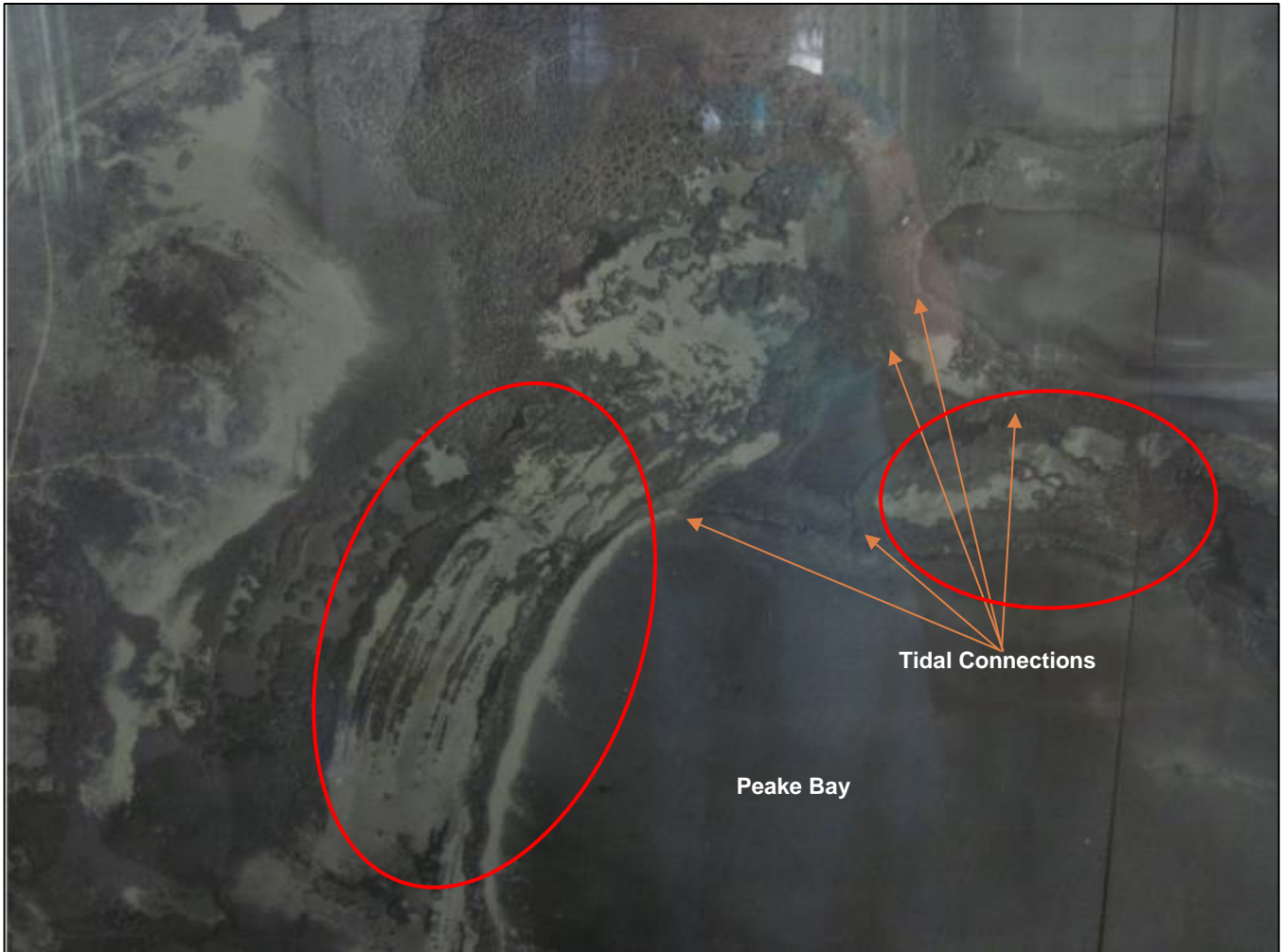
Figure 10. 1950 Aerial Showing Historic Conditions and Major Tidal Connections, Photographic Survey Company LTD.
